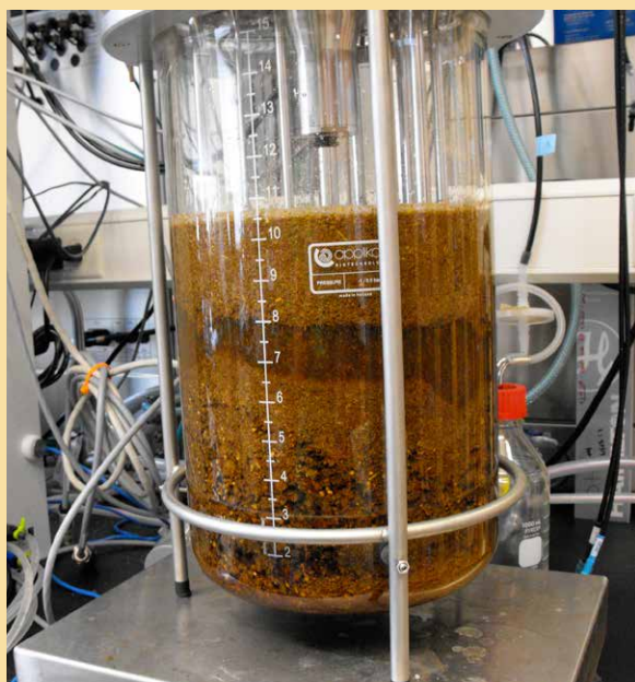
GLBRC Pretreatment Technology. AFEX TM -treated corn stover with water before enzymatic hydrolysis, a process that breaks down cellulose polymers into simple sugars using cellulase enzymes. [Image courtesy GLBRC]
