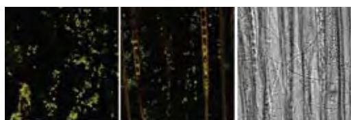
Figure 1. Fluorescent beads no fungus (left) and 3 days after inoculation with Phanerochaete chrysosporium (center). Note change in bead color with oxidation. Transmission image shows fungal hyphae (Right) Wood cellular structure is visible via auto-fluorescence (center).
