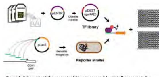
Figure 1. Schematic of the promoter hicking approach (Upper half represents the construction of the transcription factor library from identification of the clones using microarray, cloning in Gateway compatible vectors and transfer into gal4-AD vector for fusion protein expression in yeast. The lower half represents the cloning of tiled promoter fragments in fusion to the LacZ reporter and integration into yeast genome. The library and the yeast strain are then combined for 8-galactosidase monitoring assays in 96-well plates.
