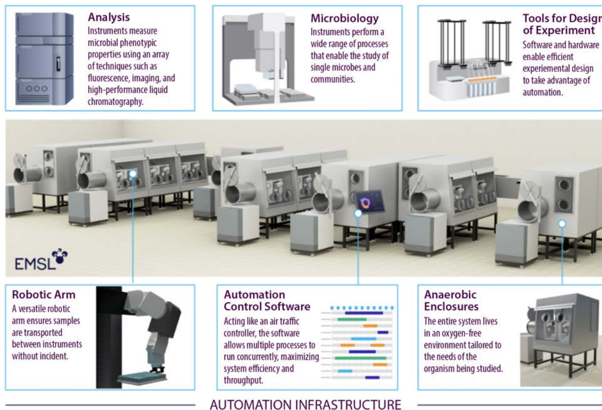
Fig. 3.2. Laboratory Automation. The Anaerobic Microbial Phenotyping Platform (AMP2) is one of many synergistic experimental user facilities supported by BER. AMP2 conducts anaerobic microbial phenotyping experiments by integrating complex devices and tools, such as robotic arms, sample transport, laboratory automation, software, and analytical instruments, all inside connected anaerobic chambers. Such studies will provide novel information about biological functions that enhance understanding, predictions, and control of complex bioeconomy-relevant processes. [Courtesy Environmental Molecular Sciences Laboratory]
