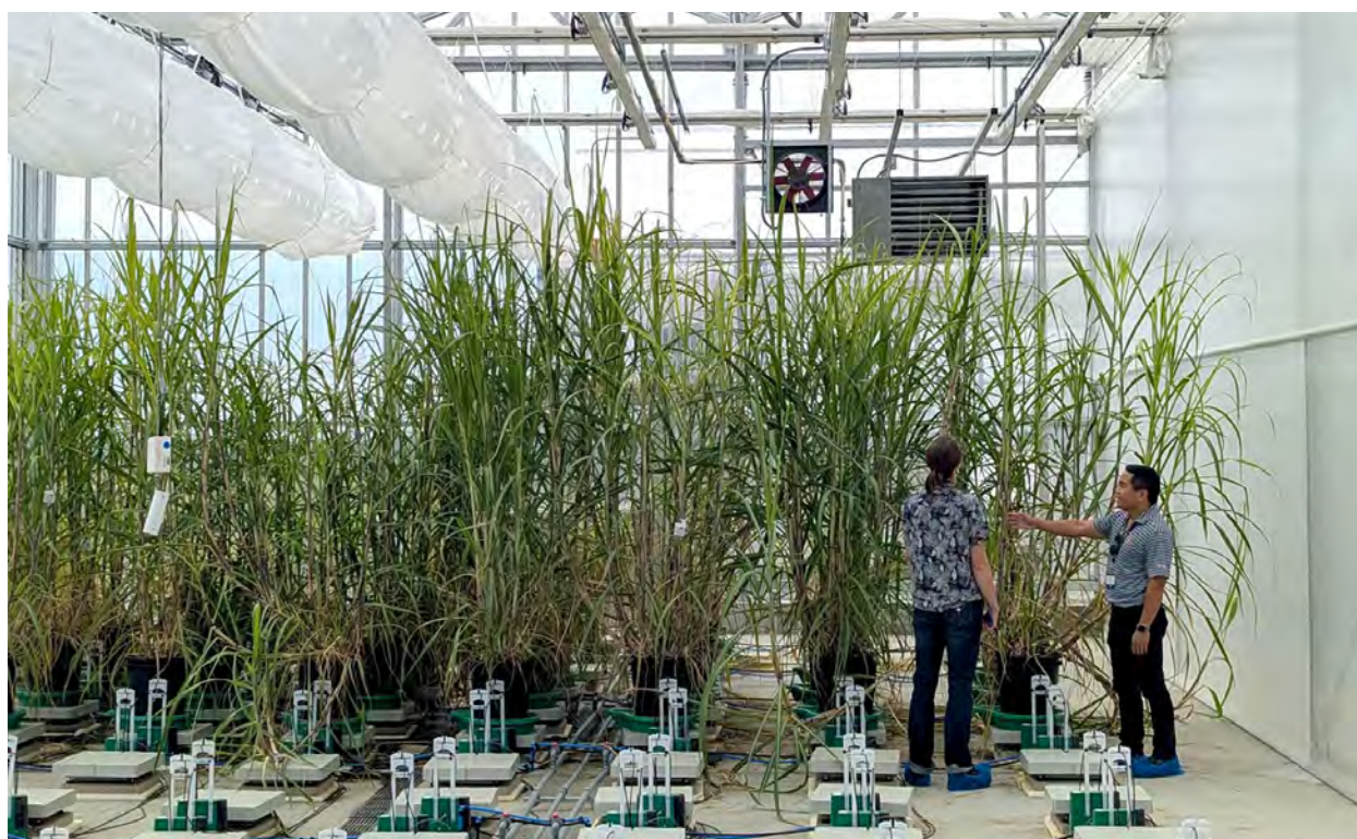
Fig. 5.5. Tall Greenhouse Facilities Can Accommodate Phenotyping of Large Bioenergy Grasses Like Sugarcane. The Plant Biology Innovation Greenhouse at the University of Illinois Urbana-Champaign was designed to accommodate high-yielding bioenergy grasses. It is outfitted with an automated lysimeter system for monitoring individual plant growth and water use, enabling high-throughput phenotyping of water-use efficiency. [Courtesy University of Illinois Urbana-Champaign]
