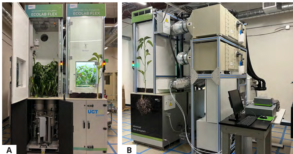
Fig. 5.4. Laboratory Ecosystems. EcoPOD growth chambers at Lawrence Berkeley National Laboratory precisely control climatic conditions to simulate field environments and support plant growth and monitoring throughout the entire life cycle ( A : two identical units sit side-by-side with doors open on the left chamber). EcoPODs are equipped with a bottom soil unit containing stainless steel lysimeters (visible inside open black cabinet) with sampling ports, soil moisture and temperature regulators, and real-time monitoring sensors. An aboveground growth chamber ( A : see plants visible inside) provides programmable LED lighting and humidity and temperature control. The growth chamber is connected to a gas analyzer ( B : see gray boxes on table next to computer) for continuous monitoring of gas fluxes during plant growth. [Courtesy Lawrence Berkeley National Laboratory]
