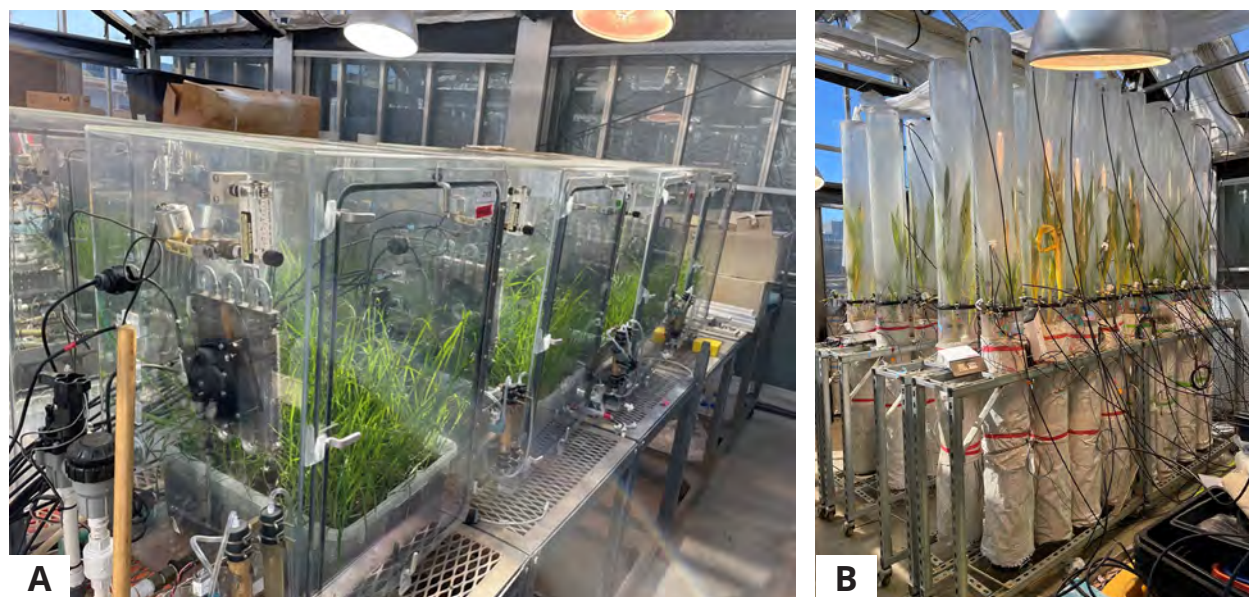
Fig. 5.3. Whole-Plant Isotope Tracing for Microbial Function Studies. (A) Wild oat ( Avena barbata ) and oil sorghum ( Sorghum bicolor ), a transgenic elevated oil line produced by the Center for Advanced Bioenergy and Bioproducts Innovation; Park et al. 2024) are grown at the Environmental Plant Isotope Chamber Facility in Berkeley, Calif. This fabricated ecosystem facility supports replicated whole-plant carbon-13-labeled carbon dioxide ( ^{13}\text{CO}_2 ) isotope tracing studies under controlled light, humidity, and temperature conditions. Carbon may be quantitatively tracked from the atmosphere into plant tissues, root deposits, soil microorganisms, and mineral associations. (B) A custom sensor relay system monitors and dynamically adjusts headspace \text{CO}_2 and ^{13}\text{C} isotope concentration. [Courtesy Lawrence Livermore National Laboratory]
